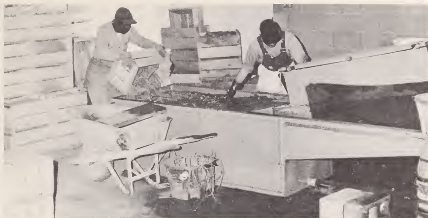
FIGURE 2.—A box of sweetpotatoes is dumped into a tank of water. Water from the washer flows through the tank and carries away the lightest silt; the tank is drained and flushed periodically to remove soil and other debris that collects in the bottom.
